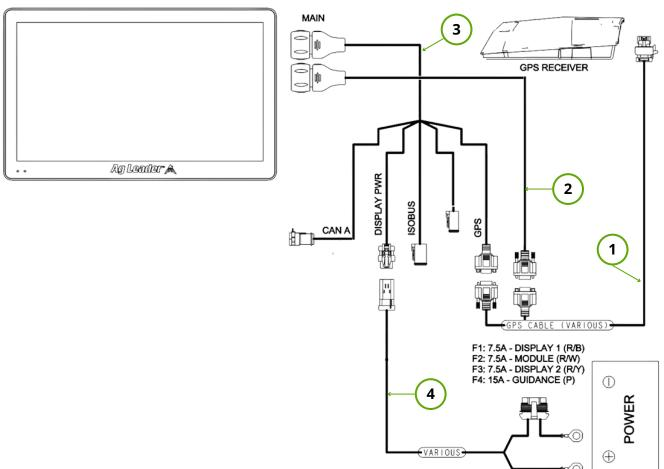
To map with a walking cart or utility vehicle, purchase the 4 cables below. The display and GPS Receiver can be removed from the sprayer and used for mapping.
